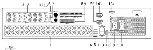
The rear panel of AR704-32 provides 32 video input interfaces.
